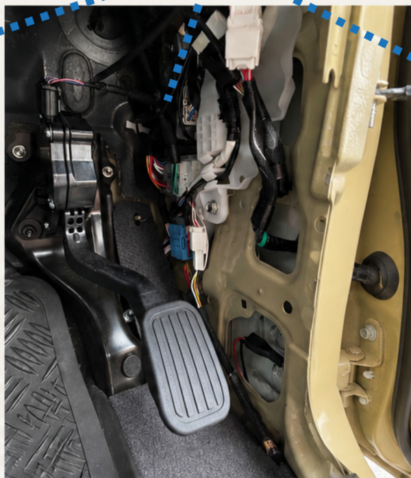
2. AFTER REMOVING KICK PANEL
