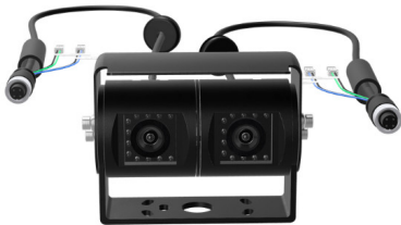
Heavy Duty Twin Camera 60° + 120° Dual View
